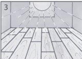
Install the panels parallel to the main light source; if there is no exterior light source, install the panels parallel to the longest wall.
