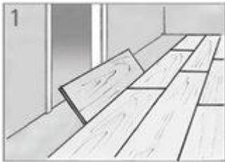
Some long edge joints cannot be installed using a 20° angle
