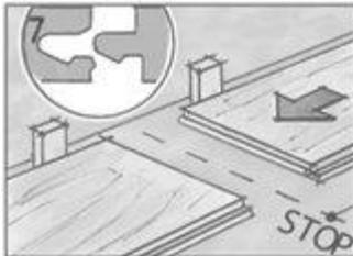
Lay the panels close together on the floor but do not lay them up against the wall yet.
